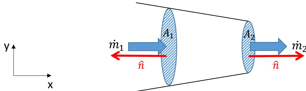
Mass flow rate inlet + mass flow rate outlet = accumulation rate (which is zero because we are at steady state)
