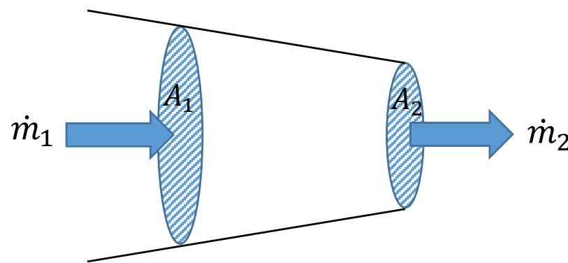
$$\text{Mass flow rate } \dot{m} = \frac{\text{mass of fluid}}{\text{time}} = \rho Q = \rho A v \quad \left[ \frac{g}{s} \right] \left[ \frac{Kg}{min} \right]$$
