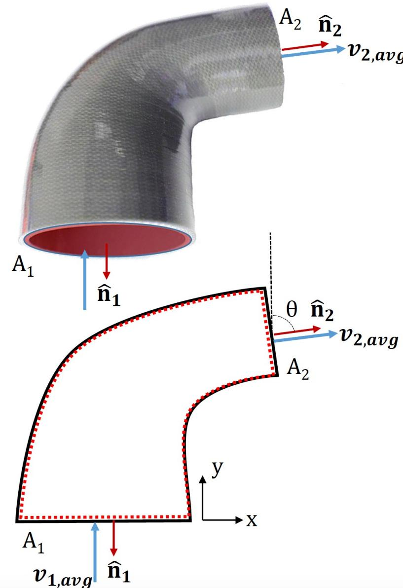
Water (50 kg per second at 80°C and a pressure of 1.5 bar) enters a reducing elbow joint. Estimate the force that the elbow joint exerts on the fluid.
