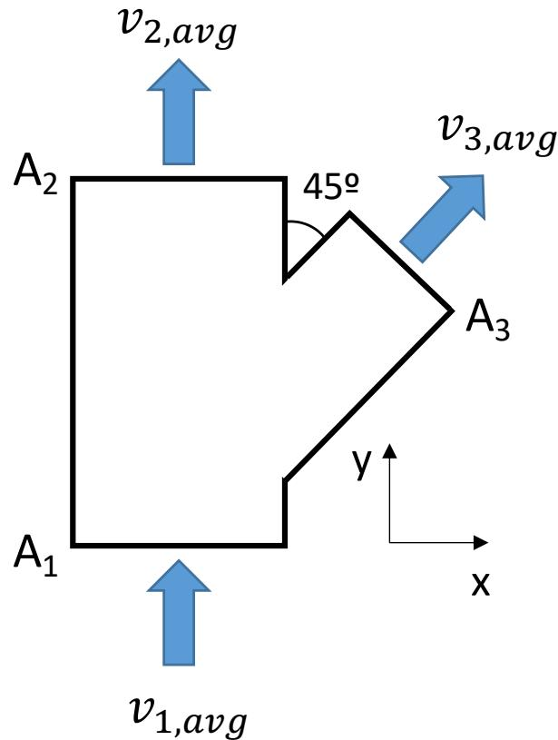
Data: water at 20°C (assume  $\rho=\text{const}$ ) flowing in the directions indicated by the arrows
