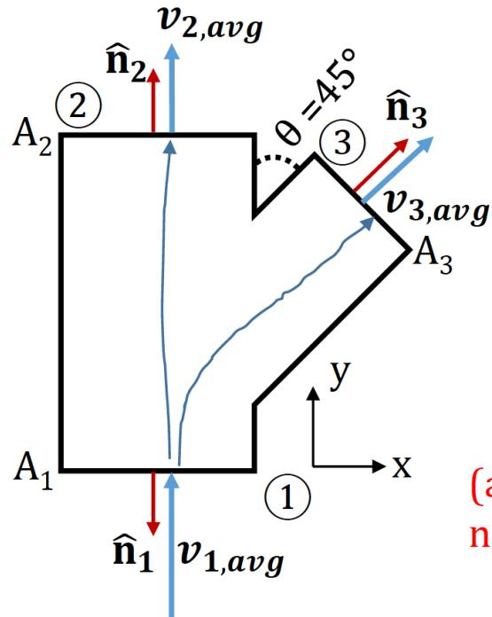
Data: system flowing water at 20°C (assume  $\rho = \text{const.}$ ),
