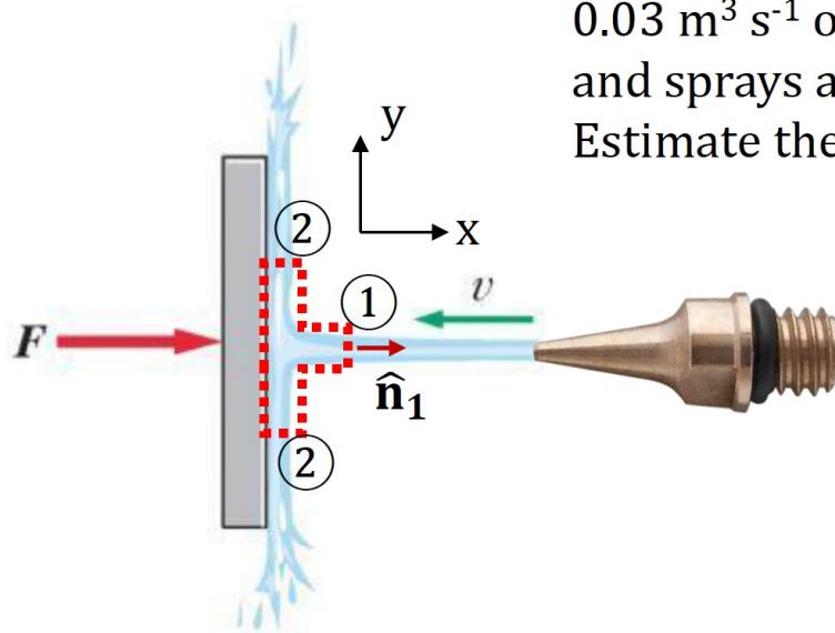
0.03 m<sup>3</sup> s<sup>-1</sup> of water at 20°C is shot out of a nozzle at 30.5 m s<sup>-1</sup> and sprays at a flat plate perpendicular to the jet. Estimate the force needed to hold the plate motionless.
