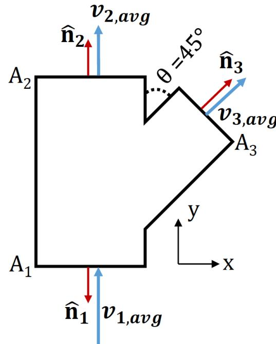
Data: system flowing water at 20°C (assume  $\rho = \text{const.}$ ),
