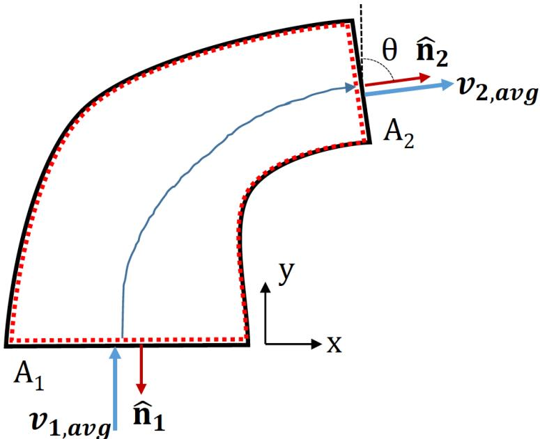
Water (50 kg per second at 80°C and a pressure of 1.5 bar) enters a reducing elbow joint. Estimate the force that the elbow joint exerts on the fluid.
