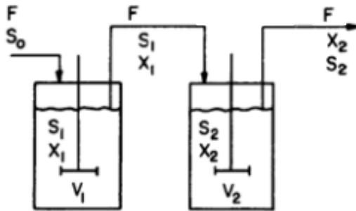
Consider a system consisting of two reactors as shown above. If the flowrate ( $F$ ) is 100 l/h, input substrate concentration is 10 g/L ( $S_0$ ), Max yield 0.5 g cell mass/g substrate, and Monod growth parameters are:  $\mu_m = 1 \text{ h}^{-1}$  and  $K_s = 0.75 \text{ g/L}$ , predict the outlet concentrations of the cell and substrate plus specific growth rate under following assumptions:
