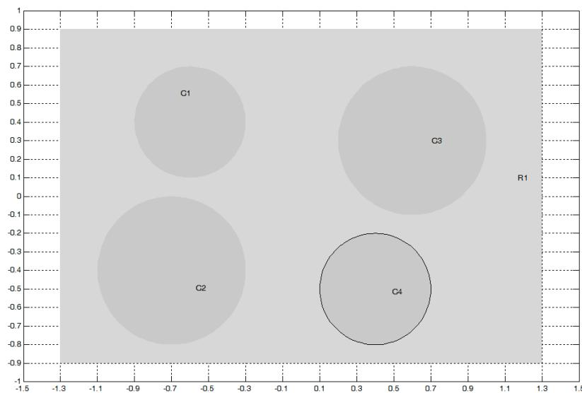
At time  $t = 0$  ( $T_0 = 20^\circ\text{C}$ ) you turn all 4 (or some, you choose) metal heater plates on with a power of  $50000 \text{ W/m}^3$ . Heat is conducted from the metal heaters to the glass plate in the x-y-plane, but we will also consider that convective heat transfer occurs to the air of the room in the z-direction (assume the convective heat transfer coefficient  $h=25 \text{ W/m}^2\text{K}$ ) and the external temperature of the room is  $20^\circ\text{C}$ .
