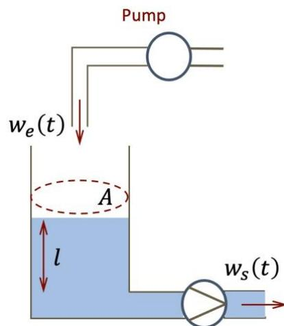
The following quantities are known: the water density  $\rho = 1000 \text{ kg/m}^3$ , the cross-section of the tank  $A = 2 \text{ m}^2$ , the output mass flow  $w_s(t) = 600 \text{ kg/s}$ , and the initial volume of the water in the tank  $V(0) = 3 \text{ m}^3$ . The measured values of the input mass flow,  $w_e(t)$ , are provided in the table below:
