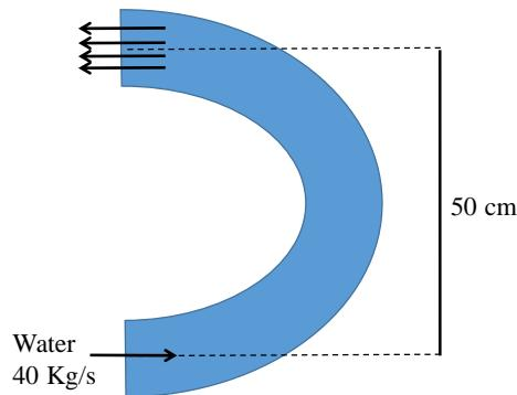
A  $180^\circ$  elbow is used to direct water flow upward at a rate of  $40 \text{ Kg/s}$ . The diameter of the entire elbow is  $10 \text{ cm}$ . The elbow discharges water in the atmosphere. The elevation difference between the centers of the exit and the inlet of the elbow is  $50 \text{ cm}$ . The weight of the elbow is  $2 \text{ kg}$ . Determine the gauge pressure at the inlet of the elbow and the anchoring force needed to hold the elbow in place.
