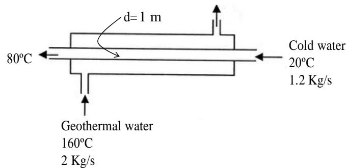
A counter-flow double pipe heat exchanger has to heat water from  $20^\circ\text{C}$  to  $80^\circ\text{C}$  at a rate of  $1.2 \text{ Kg/s}$ . The heating is to be accomplished by geothermal water available at  $160^\circ\text{C}$  at a mass flow rate of  $2 \text{ kg/s}$ . The inner tube is thin walled and has a diameter of  $1 \text{ m}$ .
