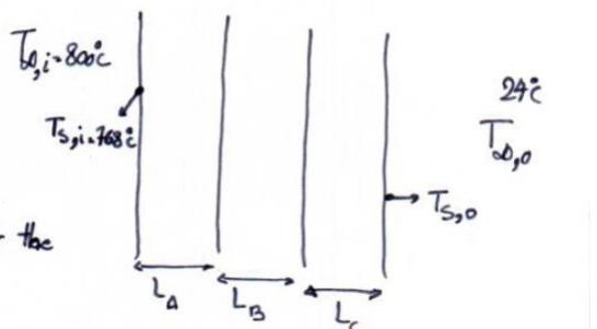
$$\frac{1}{U} = \frac{\Delta T}{\frac{Q}{A}} = \frac{768.24}{800} = 0.93 \text{ m}^2\text{K} / \text{W}$$
