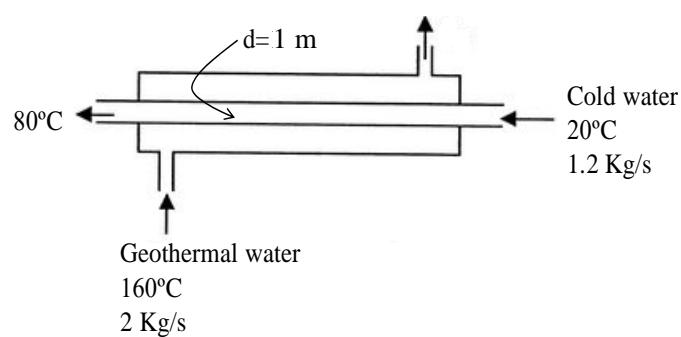
A counter-flow double pipe heat exchanger has to heat water from 20°C to 80°C which is flowing at a mass flow rate of 1.2 Kg/s. The heating is to be accomplished by geothermal water available at 160°C at a mass flow rate of 2 kg/s. The inner tube is thin walled (means that the thermal resistance is negligible) and has a diameter of 1 m.
