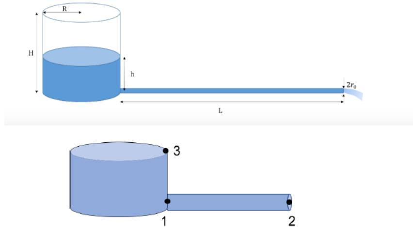
Point 1 is at the inlet of the pipe and point 2 is just the outlet. Point 3 indicates the top of the water level in the tank.
