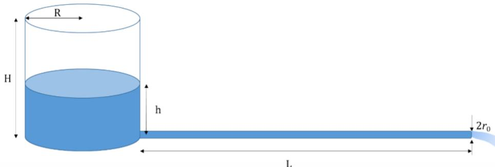
Note. While solving the exercise, you will need to make a first approximation for the velocity. You can consider the maximum possible velocity, which is the one you get assuming  $h=H$  and the friction coefficient being the minimum possible considering your  $\epsilon/D$  in the Moody diagram.
