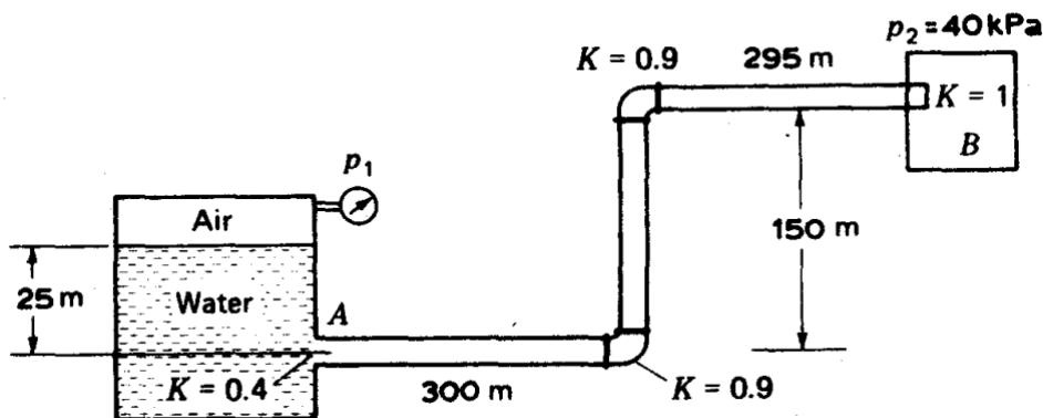
Note: Keep in mind that a streamline can be maintained all the way from point 1 (water surface) to point 2 (B)
