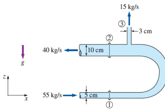
At flange 1, the total absolute pressure is 200 kPa, and 55 kg/s flows into the pipe. At flange 2, the total absolute pressure is 150 kPa. At location (3), 15 kg/s of water discharges to the atmosphere, which is at 100 kPa. **Determine the total x-force and z-force at the two flanges connecting the pipe.** Consider frictionless flow.
