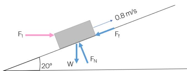
With the friction force parallel to the surface, the normal force perpendicular to the surface and the weight in the direction of gravity acceleration.
