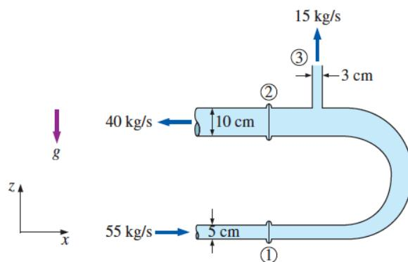
At flange (1), the total absolute pressure is 200 kPa, and  $55 \text{ kg/s}$  of water flows into the pipe. At flange (2), the total absolute pressure is 150 kPa, and water flows at  $40 \text{ kg/s}$ . At location (3),  $15 \text{ kg/s}$  of water discharges to the atmosphere, which is at 100 kPa. Determine the total x-force and z-force at the two flanges connecting the pipe. Consider frictionless flow and neglect volume forces.
