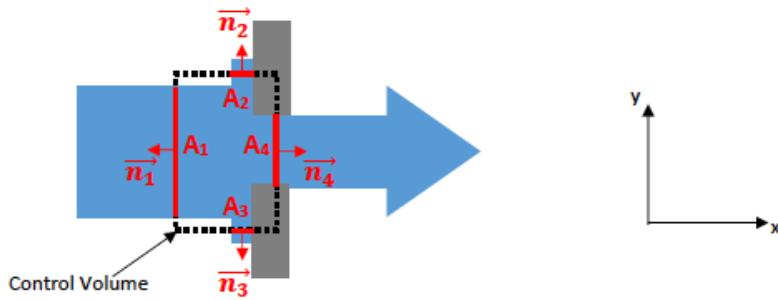
In this system, all the fluid is at atmospheric pressure, therefore the sum of the forces applied on the control volume is equal to 0. Moreover, if we neglect the gravitational and friction forces, the momentum balance gives :
