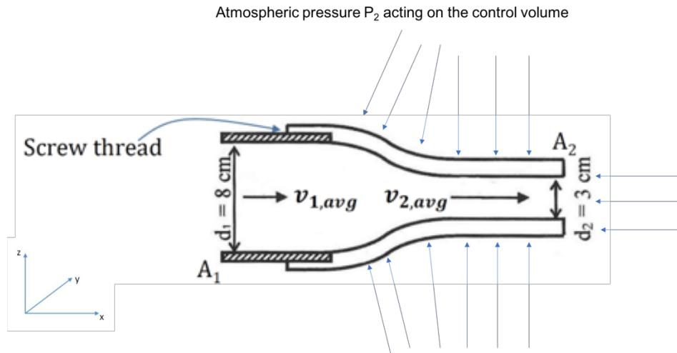
Hence we need to consider an area  $A_2^*$  for the atmospheric pressure  $P_2$  and not just  $A_2$ . Due to the irregular shape of the control volume,  $P_2$  is acting on every elemental area in a different direction.
