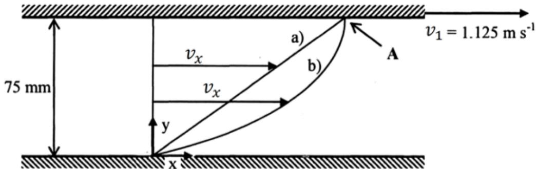
A plate moves with a constant speed of  $v_1 = 1.125 \text{ m s}^{-1}$  on top of another plate which is stationary. The two plates are spaced 75 mm apart and a Newtonian fluid ( $\mu = 0.048 \text{ Pa s}$ ) fills the space between. Estimate the shear stress at the wall and at the stationary points 25 mm and 75 mm from the stationary wall, in the case of:
