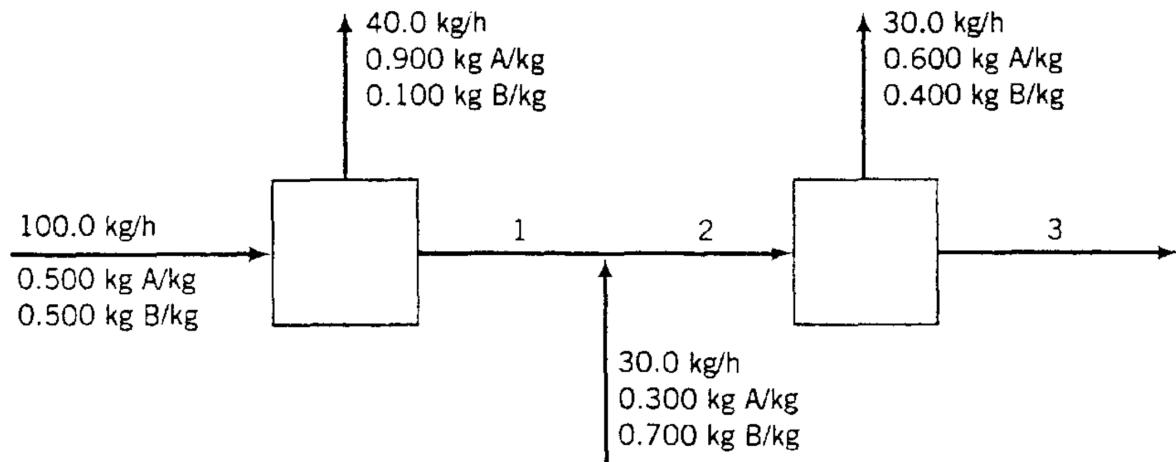
Calculate the unknown flow rates and compositions of streams 1,2, and 3.
