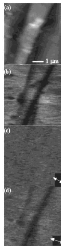
Figure 21. NSOM (a) topography, (b) total photoluminescence, and (c, d) polarized photoluminescence of a stretch-oriented PPV film. Comparing the total photoluminescence image (b) with the topography image (a) shows that the photoluminescence efficiency decreases near the edges of the fiberlike features and the clusters. There is little photoluminescence observed at a polarization orthogonal to the stretch axis of the fibers as shown in (c). Reproduced with permission from ref 81. Copyright 1997 Elsevier Science.
