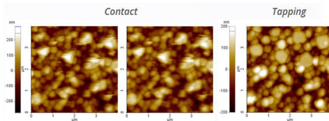
↳ This series of pictures highlights the strong effect of the lateral forces that distort the cantilever and thus degrade the lateral resolution when running the AFM analysis in contact mode.
