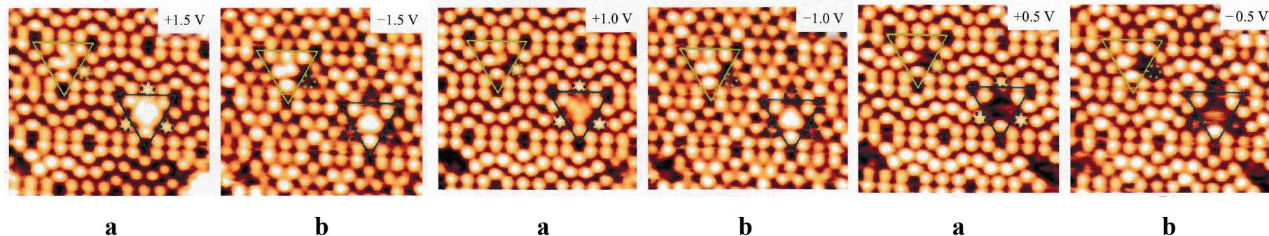
empty **a** and filled **b** state STM images of Zn-induced nanocluster on an Si(111) surface. The bias voltages represent the polarisation of the sample.
