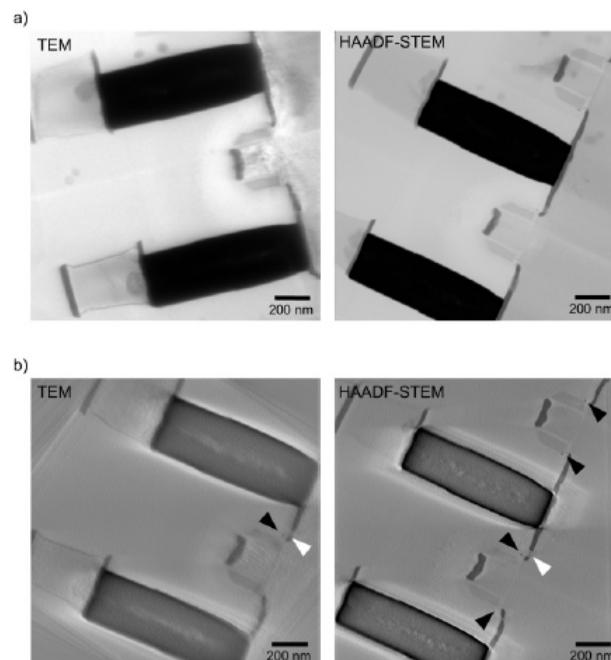
⇒ BF-TEM / HAADF-TEM images (a) and the 3D reconstructed images based on tilt series of BF-TEM / HAADF-TEM images (b) of a transistor.
