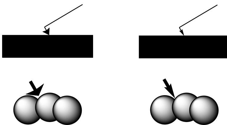
↳ An STM or AFM image comes from a convolution between the surface topography and the tip shape as described on the scheme above. The tip shape must be studied by SEM prior to any experiment to get the real vertical and lateral resolutions of the microscope.
