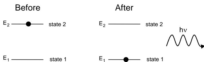
In a third type of process, the molecule initially in the excited state encounters a photon with energy equal to the separation between states 1 and 2. In this case, the photon can induce or stimulate a downward transition from state 2 to state 1.
