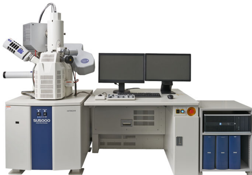
Fig. 1.15 Hitachi-SU5000 scanning electron microscope. This instrument uses a Schottky-emission source and provides a resolution of 1.2 nm at an accelerating voltage of 30 kV or 3 nm at 1 kV (2 nm in deceleration mode). Variable pressure mode (10–300 Pa) is an option
