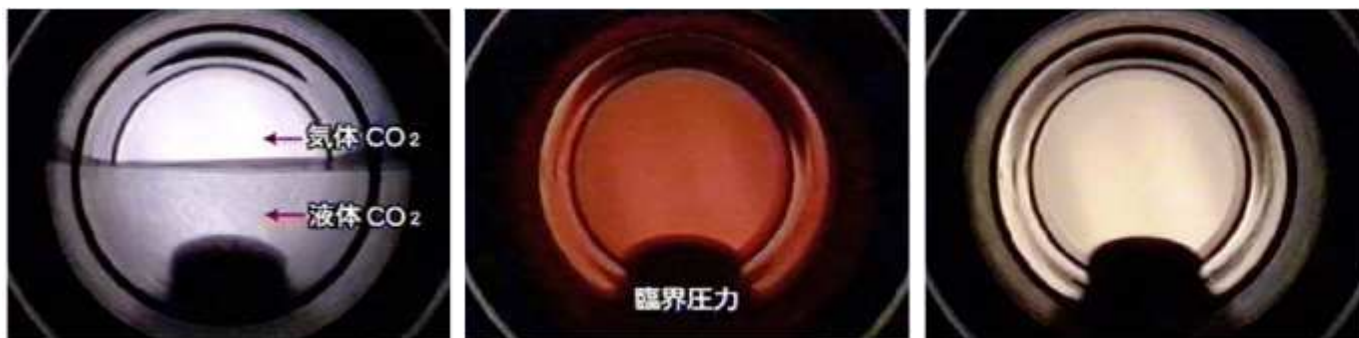
Image 2: CO 2 in different states of matter, from left to right: gaseous/liquid; at supercritical point (Rayleigh-scattering); in supercritical state
