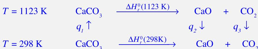
$$\Delta H_r^0(T = 1123 \text{ K}) = -q_1 + \Delta H_r^0(T = 298 \text{ K}) - q_2 - q_3$$
