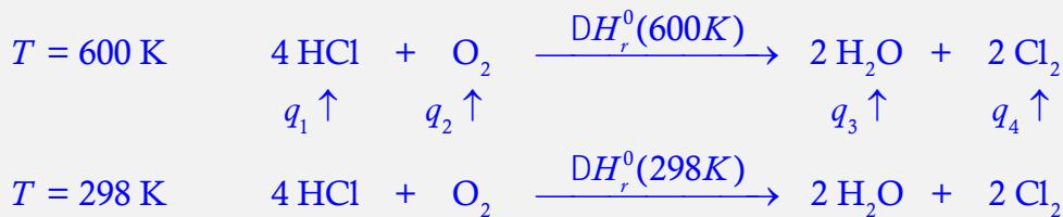
$$q_1 + q_2 + \Delta H_r^0(600\text{ K}) = \Delta H_r^0(298\text{ K}) + q_3 + q_4$$
