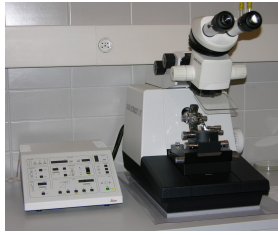
Resin embedded tissue block/ultramicrotome - for block preparation and sectioning
