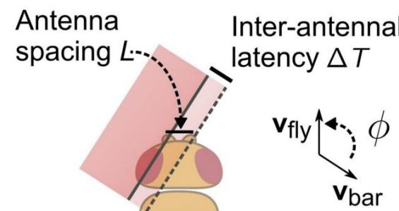
$$\Delta T = \frac{L \sin \phi}{|\mathbf{v}_{\text{bar}}| - |\mathbf{v}_{\text{fly}}| \cos \phi}$$
