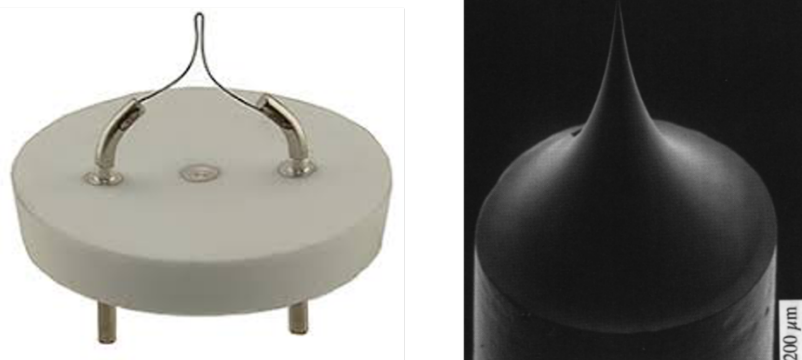
Figure 3. Different types of EM emitters: thermal emission (left) and field emission (right).
