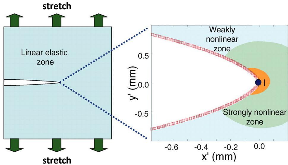
SOURCE: Livne A, Bouchbinder E, Svetlizky I, Fineberg J (2010) The near-tip fields of fast cracks. *Science* 327(5971): 1359-1363 PMID:20223982.
