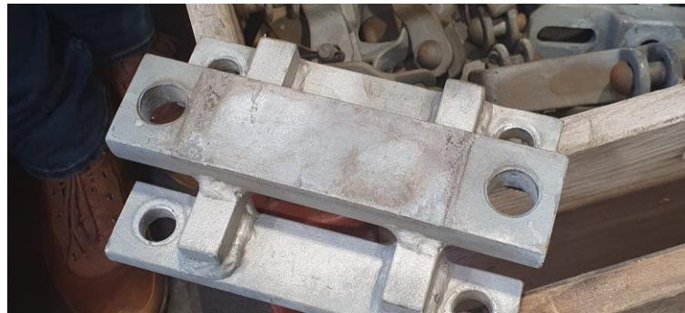
Refurbishment of catenary material – "as good as new". High savings potential for standardised parts. Scale to all assets.
