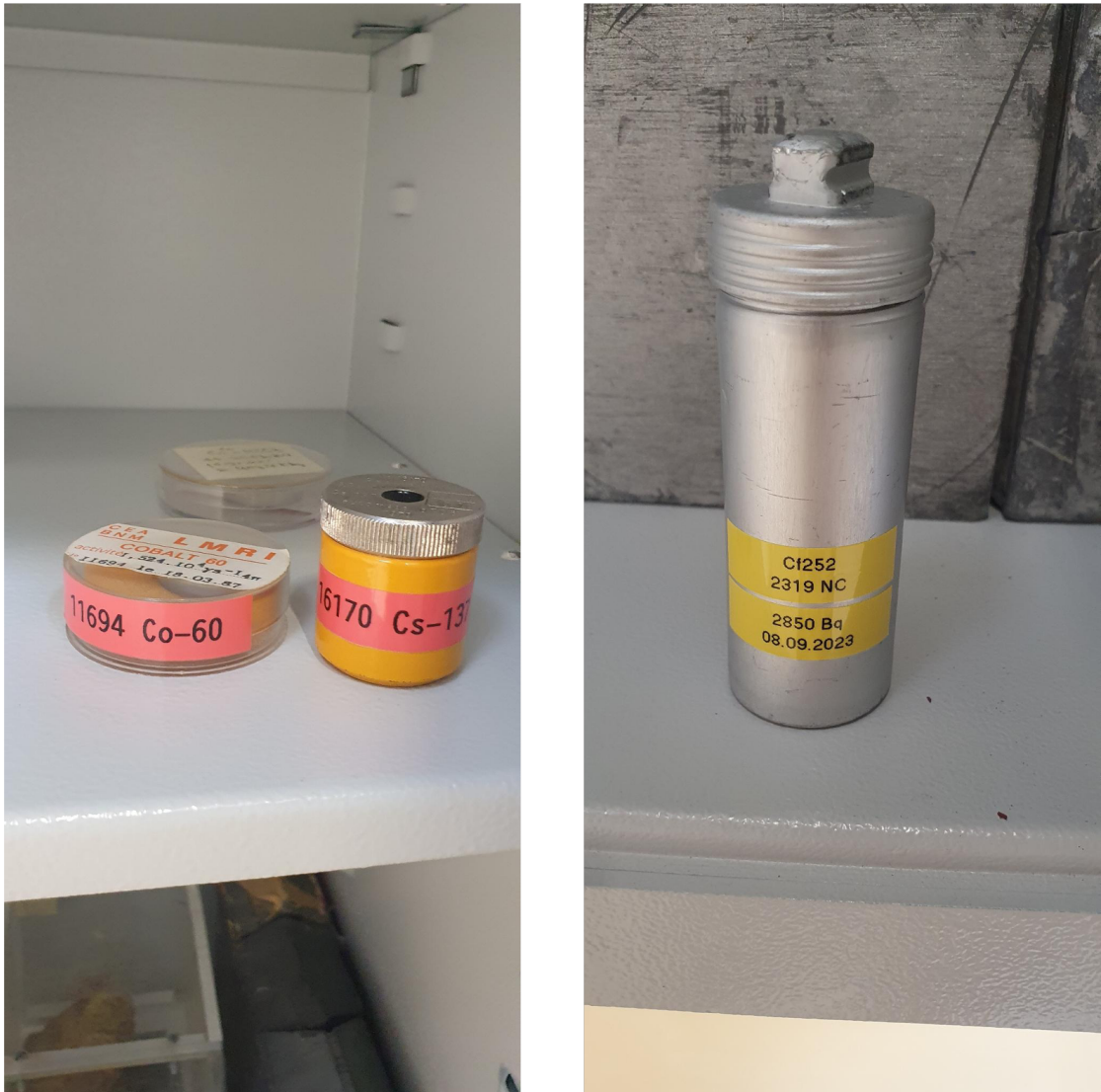
Figure 6.5: Left: Co60 and Cs137 sources to be used for the experiment. Right: Californium source that can be used for a neutron/gamma pulse shape discrimination experiment.
