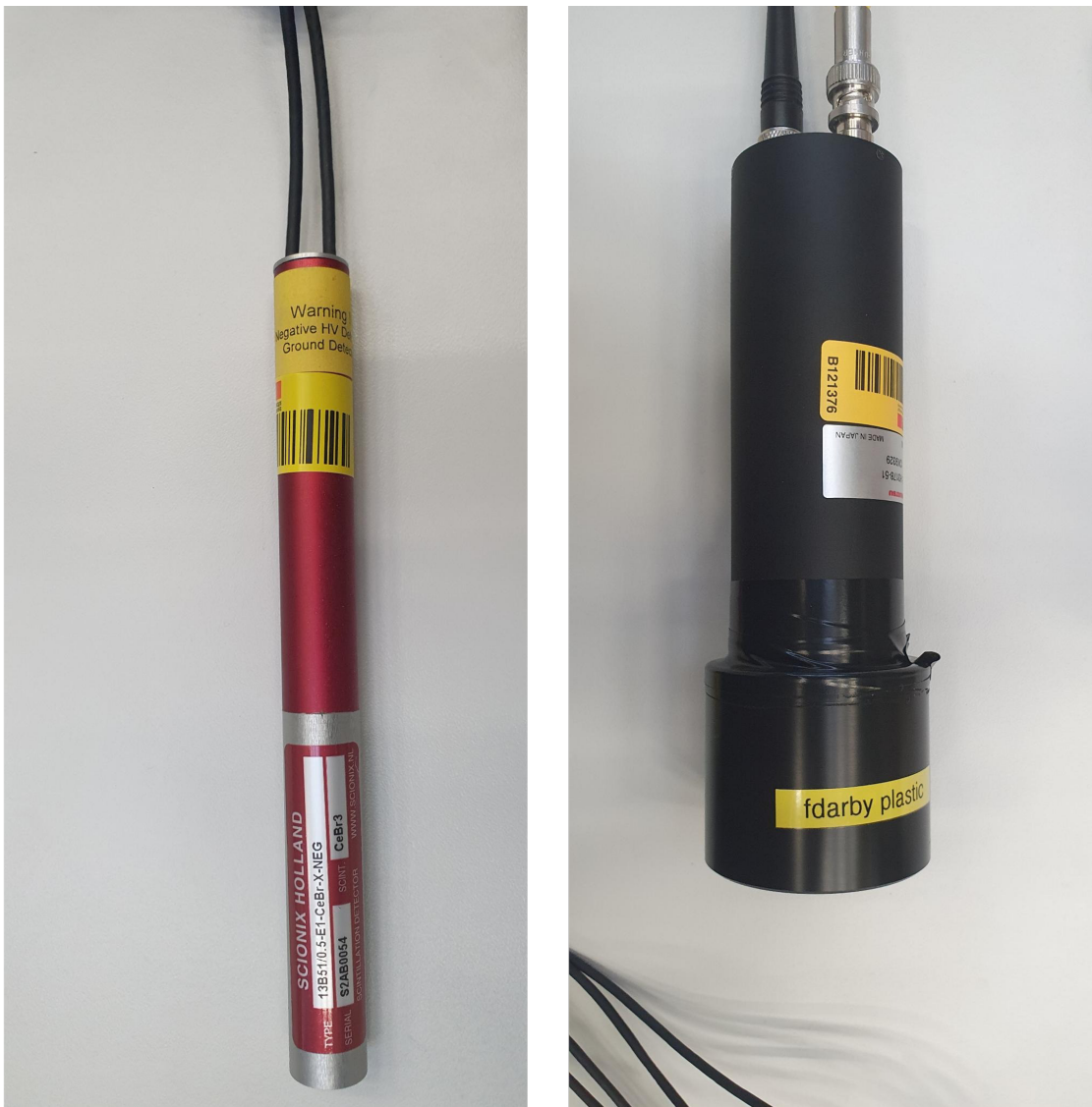
Figure 6.3: Left: Scionix CeBr3 detector. The bottom houses the crystal, the top houses a crystal. The whole detector is encased in aluminium for light tightness and mechanical protection. Right: Organic scintillator. The top part is a Hamamatsu H3178-51 PMT, the bottom is a light-tight plastic hollow cylinder that contains a plastic scintillator cylinder of 1cm height and diameter. Be careful handling these detectors, the PMTs are delicate and the crystals can easily crack!
