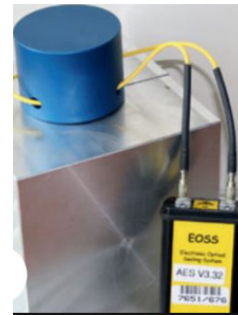
COBRA seal (single use) Fibre optic loop with verification tools (in situ verifiable)
