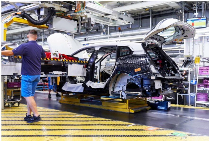
The cowl panel and rear window frame components are manufactured from continuous fibre reinforced thermoplastics (CFRTP) using an all-new method (Production at Plant Dingolfing)
