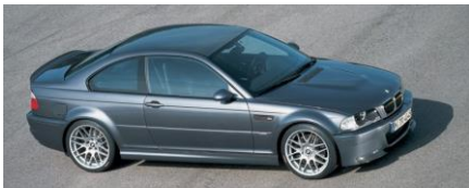
BMW's Landshut Plant 50% lighter than steel, RTM of CF/epoxy, 1800 T press
