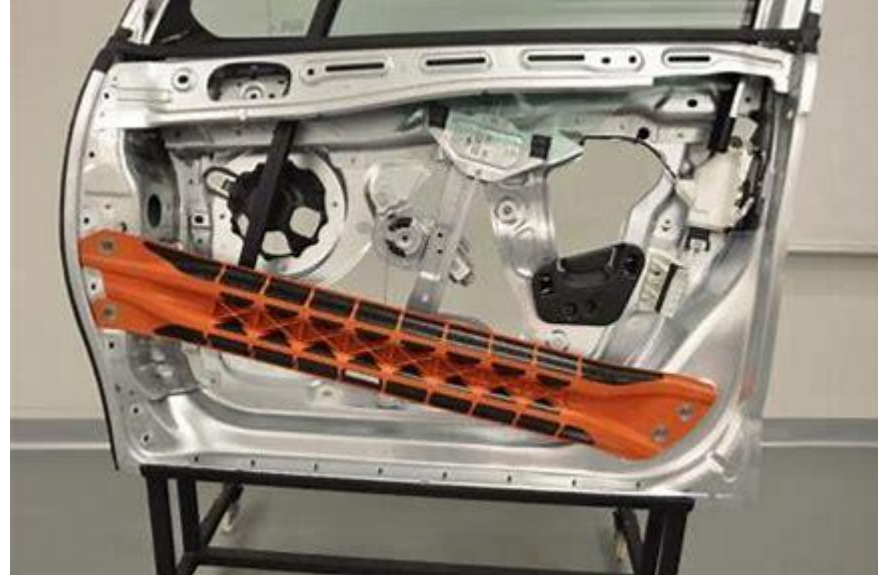
PSA Side Intrusion Beam development with overmolded DuPont Vizilon™ TPC sheet, JEC Paris, March 2013
