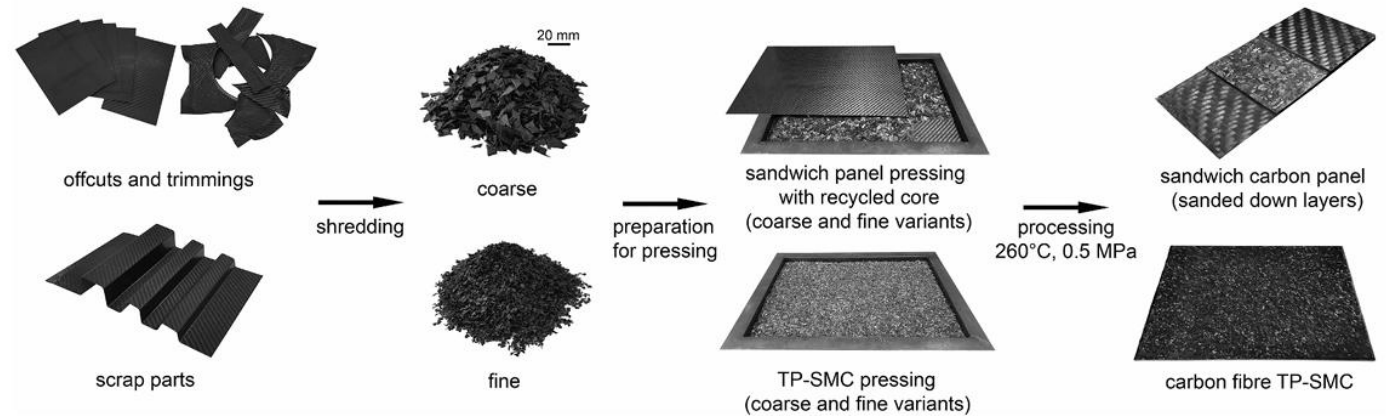
Fig. 1. Recycling routes for PP-GF and PA6-CF based TPCLs.
