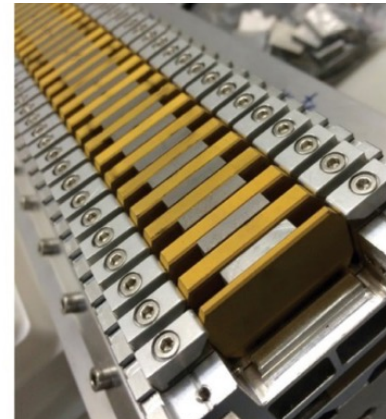
The lower magnet array of a U15 (15 mm period) undulator.
