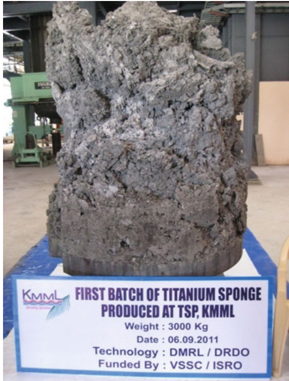
Fig. 4.6 First titanium sponge cake (weighing about 3 tons) produced in the KMML titanium sponge plant
