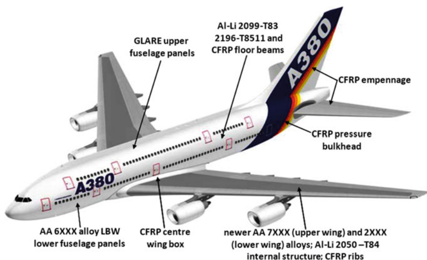
Fig. 14.3 Airframe materials distributions for the Airbus A380 [2]: AA 2XXX, 6XXX and 7XXX = conventional aluminium alloys; Al–Li aluminium–lithium alloys; LBW Laser Beam Welding [3]
