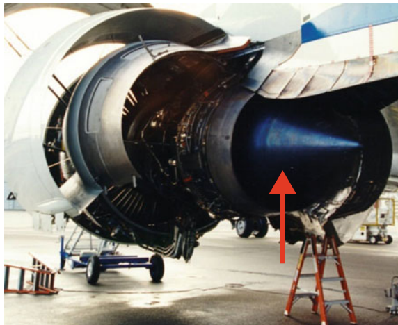
Fig. 6.25 Use of Beta 21S as an engine tail plug (indicated by an arrow)
