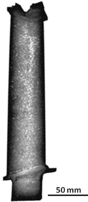
Fig. 10.7 TiAl LPT turbine blade for the GENx aeroengine. Source GE
