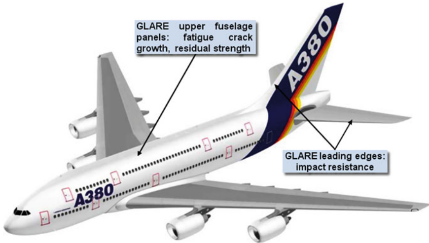
Fig. 13.3 GLARE deployment in the Airbus A380 [3–5]
