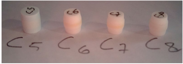
Co-fired sample (sandwich A-B-A)
