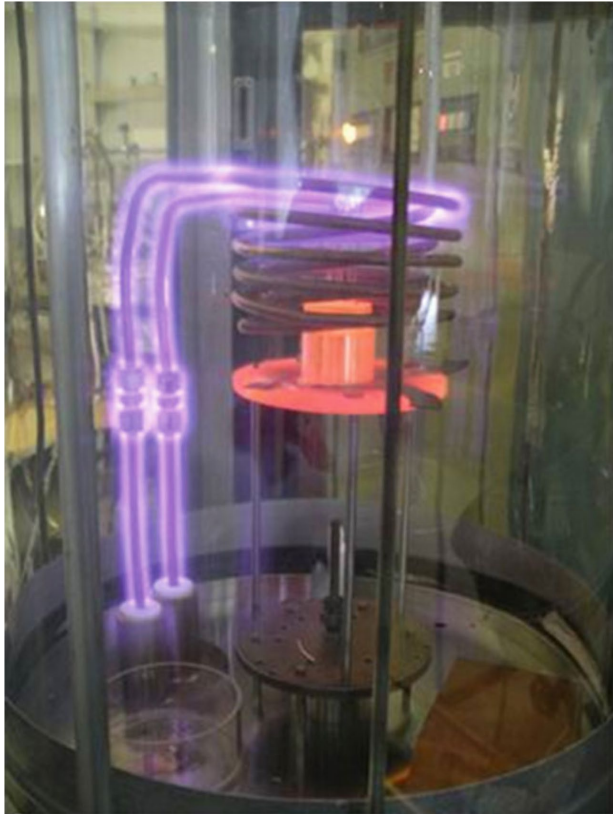
Induction furnaces at 60-1000Hz, can reach 3000°C.
