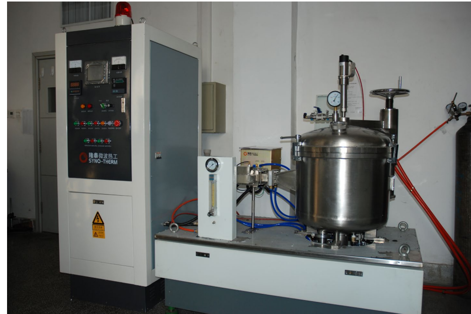
Microwave Sintering is also one kind of induction furnace. Normally working at 2.4GHz for industrial use.
