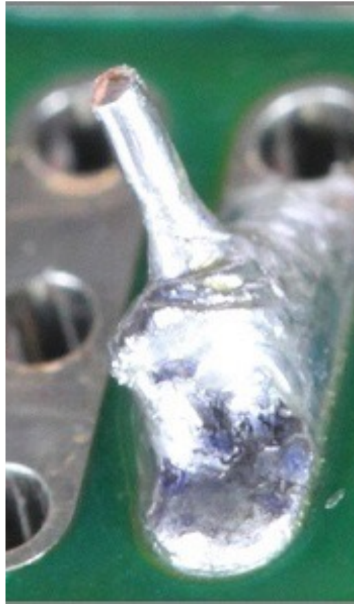
Cold solder joint
