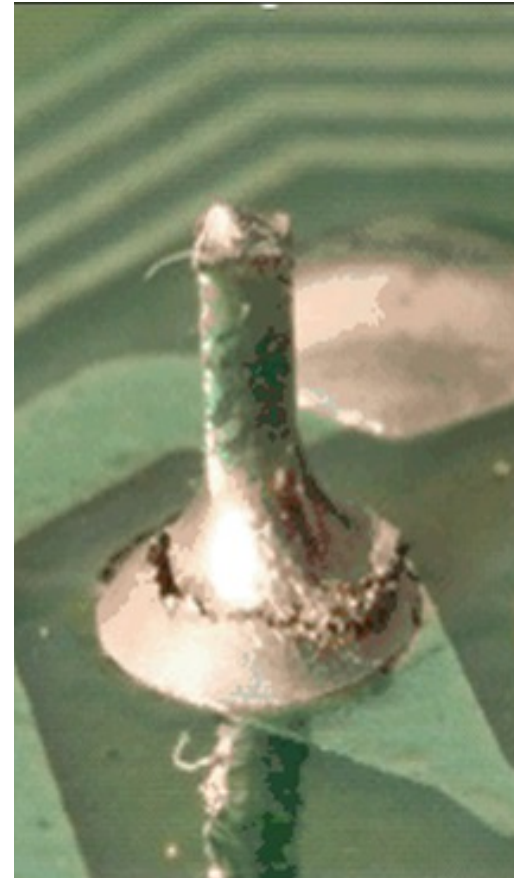
Cracked solder joint
