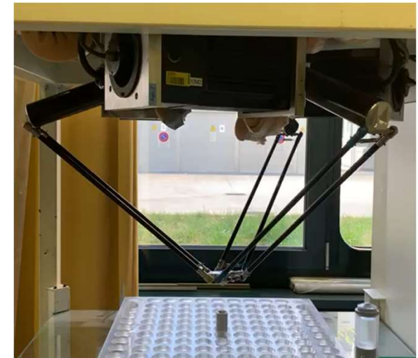
August 2019 0,4mm RMS_error @30 Ge acceleration pick_and_place
