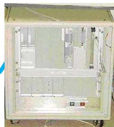
Control cabinet: • Intelligence • I/O boards for the axes, • I/O cards for safety, • Power stage,
