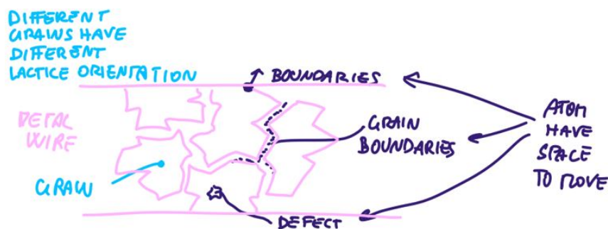
Figure 6.8: Different grains have lattice orientations.
