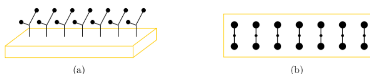
Figure 11.1: Molecular wire implementation: (a) a substrate, for example a gold nanowire, onto which molecules are placed, (b) top view.
