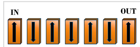
Figure 14.15: iNML inverter horizontal wire.
