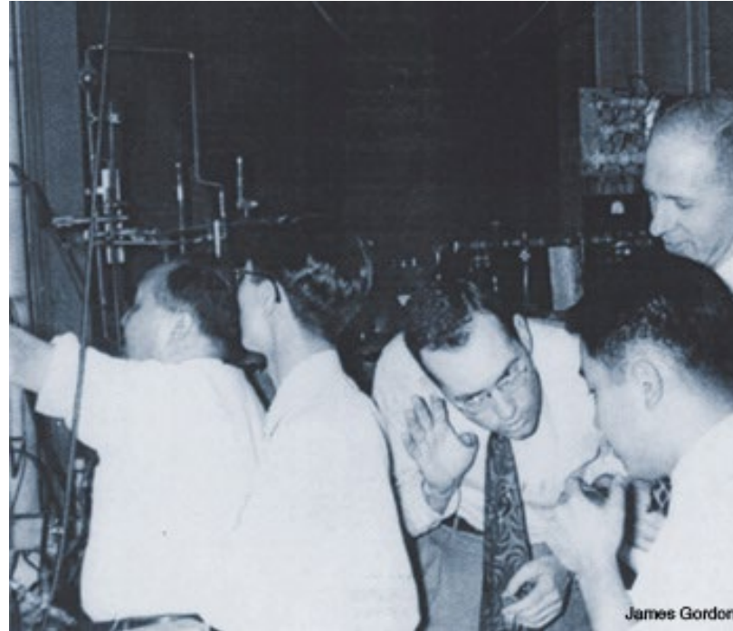
Townes listening to the 100 Hz beating produced by the interference of the first two masers
