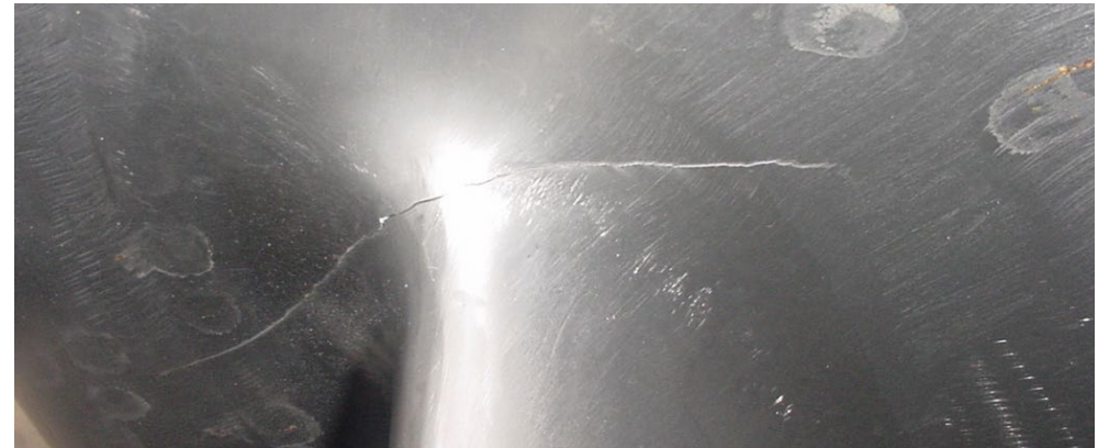
Severe erosion in pump propellers
