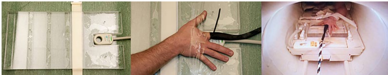
Fig 1. The radiofrequency coil inside the clear housing (left). The metocarpophaangeal (MCP) joint of interest centred over the bore of the radiofrequency coil (middle). The participant's hand within the imaging magnet (right).
