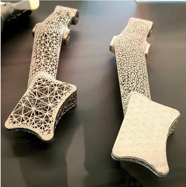
Break pedals (3D printing, Titanium) Scuderia Ferrari, Formula 1
