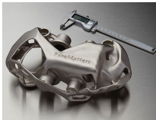
Figure 5.12: TO part with electroplating for reinforcement
