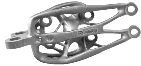
(b) Aircraft floor bracket [37]
