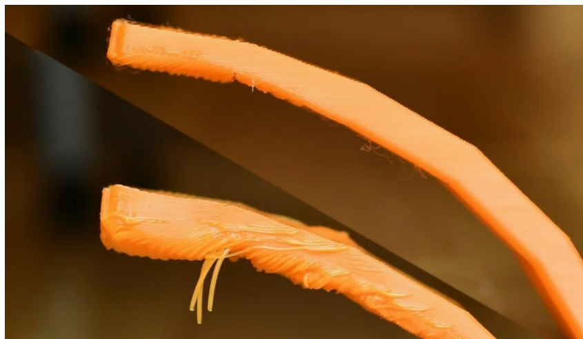
Figure 11: The same part printed with (top) and without effective cooling (bottom) shows a great difference in print quality [13].
