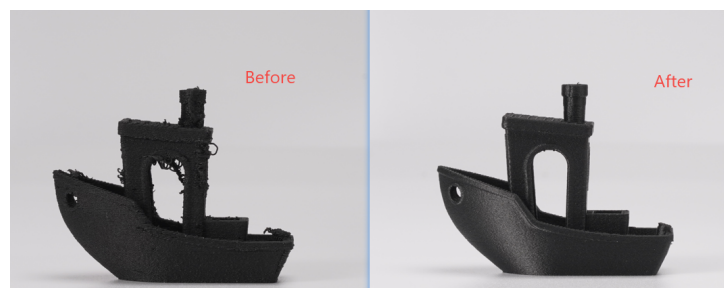
Figure 21: Effect of humidity of part quality [6].
