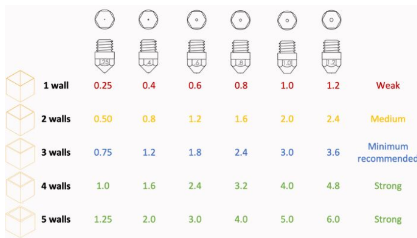
Figure 14: The minimum wall thickness can be calculated as a multiple of the printer’s nozzle diameter [26].
