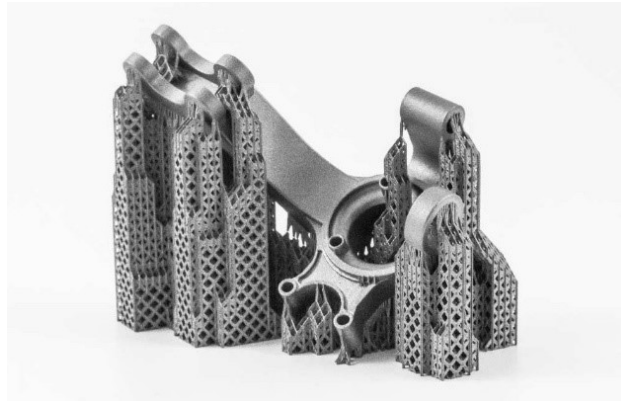
Figure 12: Use of supports in metallic AM. [29]
