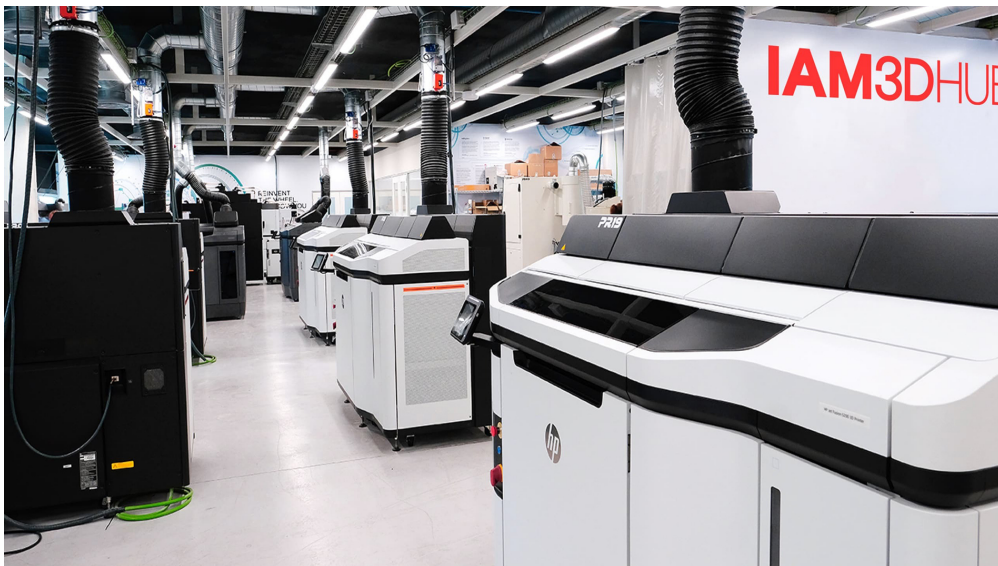
Figure 11: HP Multi Jet Fusion industrial 3D printers in IAM3DHUB facilities. [27]
