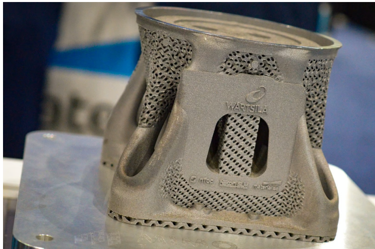
Figure 2: Wärtsilä cylinder head demonstrator [5]
