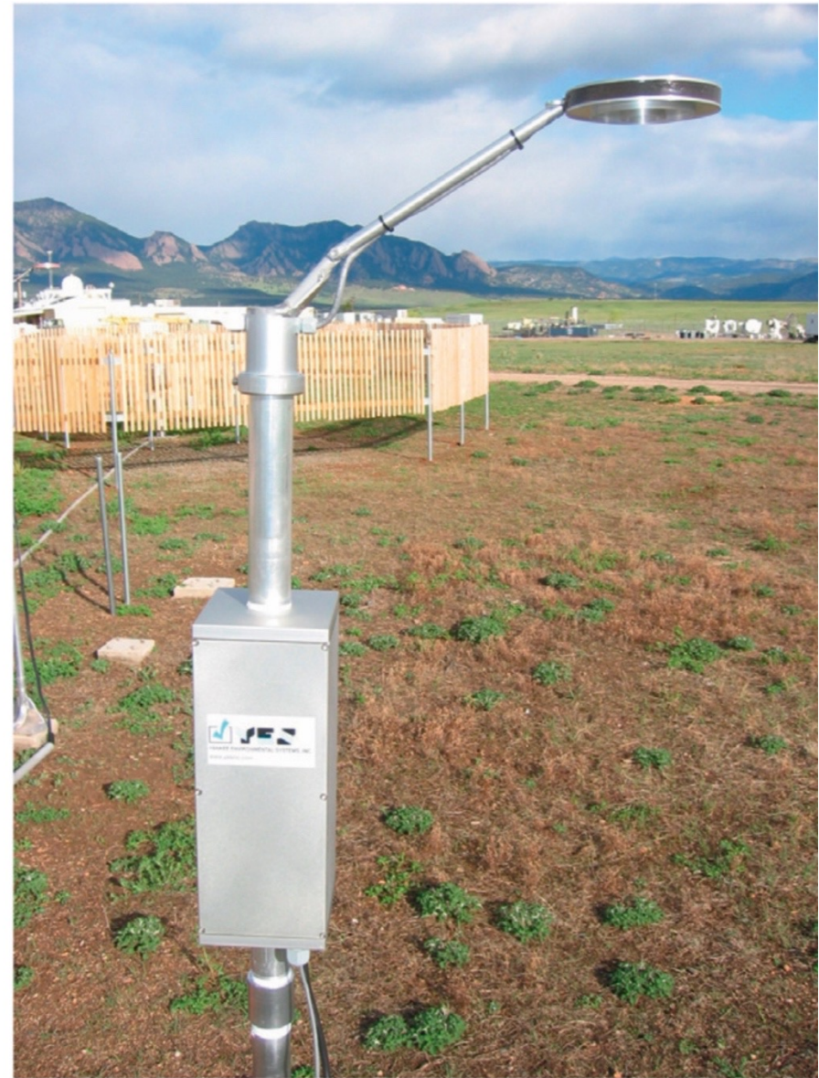
FIG. 2. Commercial version of the hotplate snow gauge from
