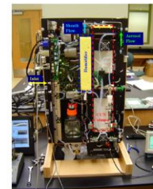
Cloud Condensation Nuclei Counter, US Patent 7,656,510
