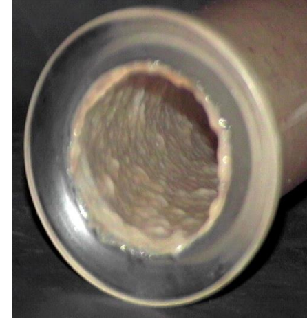
Biofouling on permeate surface of CA membrane (Water Factory 21)
