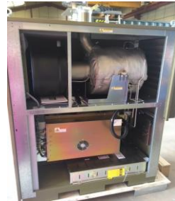
Containerised Capstone C30 Micro-turbine
