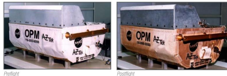
Figure 4. Preflight and postflight images of the Optical Properties Monitor shown with ultraviolet-darkened insulation after nine months of exposure on the Mir Space Station.
