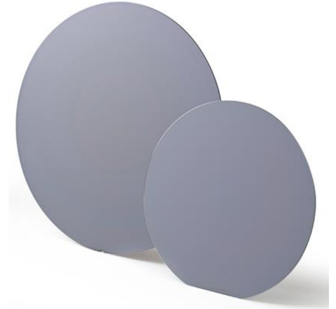
Wafers: size has grown over time. TODAY's standard: 12" (300mm)
