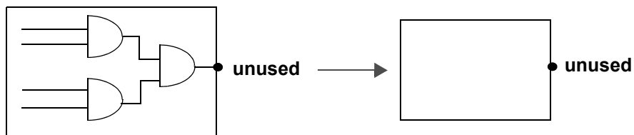
Figure 25 Minimizing Logic Driving an Unconnected Output Port
