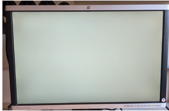
Figure 5: A successful implementation of a VGA controller should have an all white video output from the FPGA.
